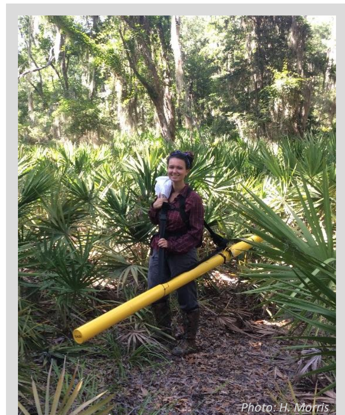
Figure 11: Dessa Dunn carrying the EMI instrument to map soil electrical conductivity, which is used to calculate an indicator of plant available soil moisture.
