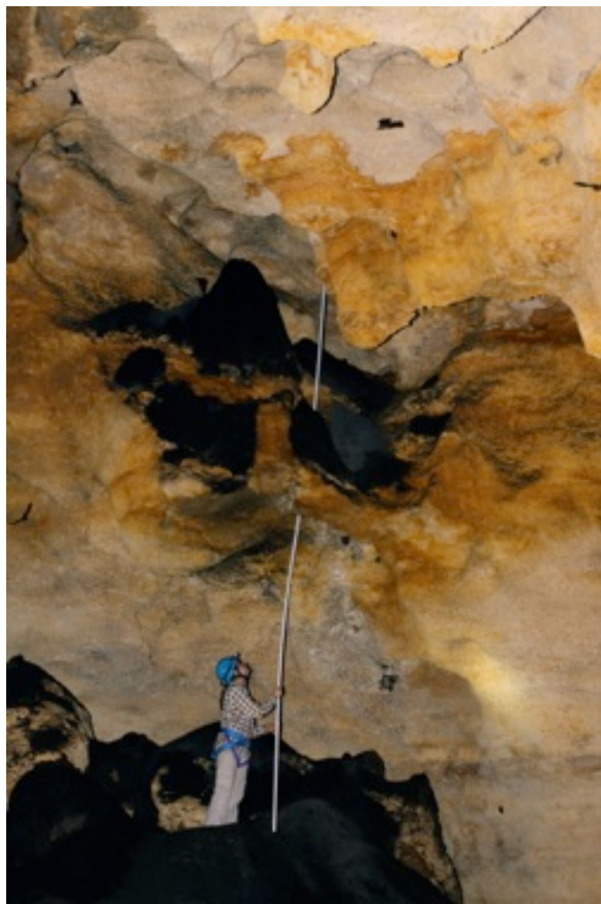
Installing a data logger to record temperature and humidity near the nursery in Bat Cave, Naracoorte. Photo: Steve Bourne
